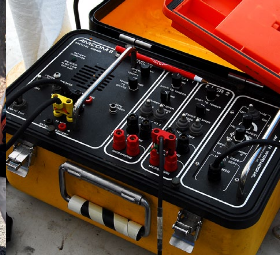
Chris Weaver (pictured left) being readied for a dive in the Mark V suit. While in the water, surface support crew are able to speak with the divers with specialized communication equipment, shown here above.
